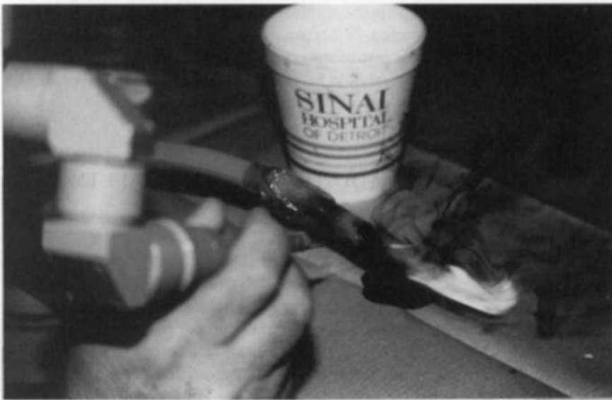
Figure 2-6. Ignition of oxygen-filled endotracheal tube results in ignition and creation of a blowtorch-like effect. Covered foot pedal.
