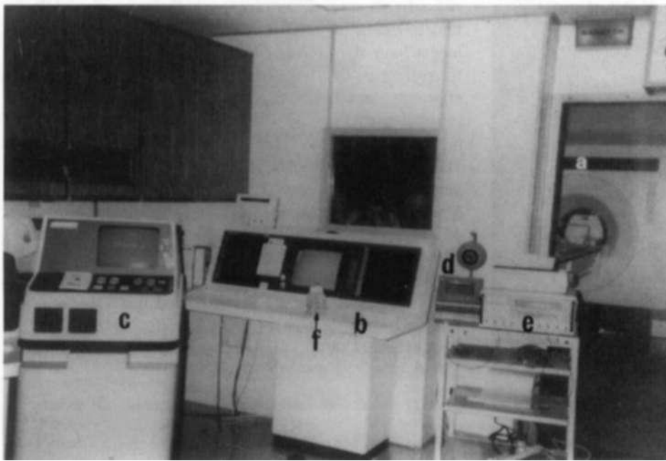
Figure 12-4. Setting of the MR suite showing the GE Signa MR magnet (A), the operator console (B), the Laser-scope KTP:YAG laser, which is kept outside the magnet (C), the Coherent power meter and detector head (D), the Luxtron fluoroptic thermometer (E).
