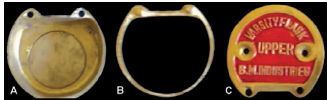
FIGURES 14.1A to C: Dental flask (A) Lower chamber (B) Middle chamber (C) Lid
